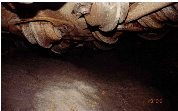
Fig. 5: Close-up of the rotary bit. The borehole diameter is 5 m. Photo E. Meier.
